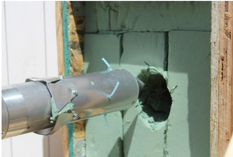
Figure 4.7: Extraction test with roots fully extended
