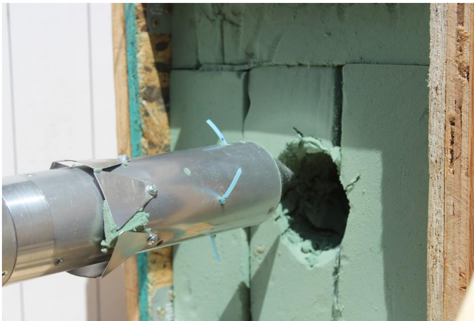
Figure 4.8: Angled impact between anchoring system and regolith
