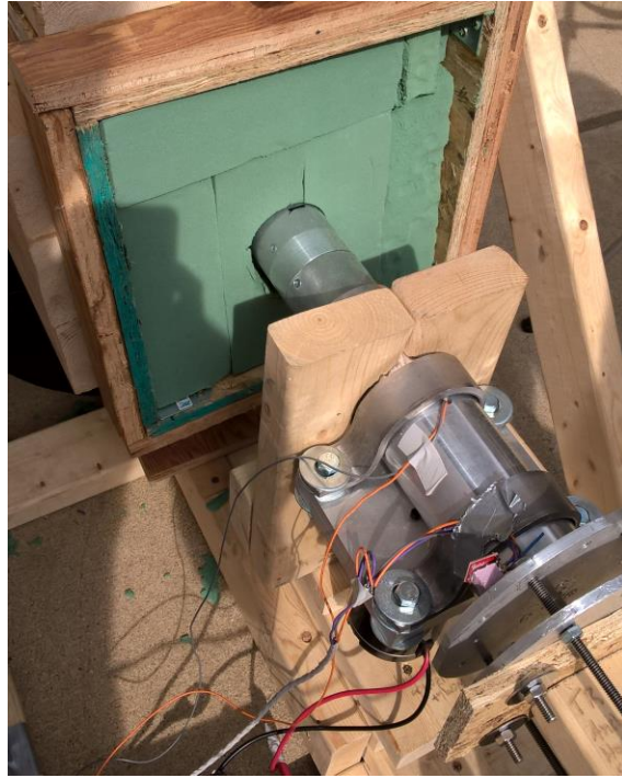
Figure 4.6: Device penetrating regolith past compliant flaps
